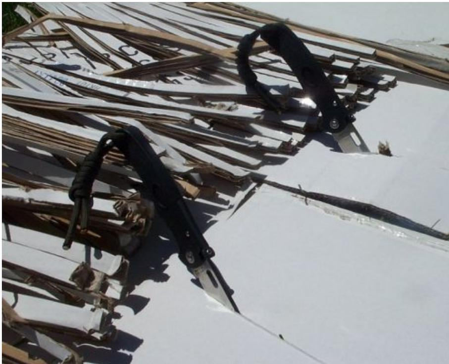
Cardboard is very hard on edges, still it took over a hundred 12 inch slices before the AUS-8 edge started to rip the outer layers indicating that the knife was finally dulling.
