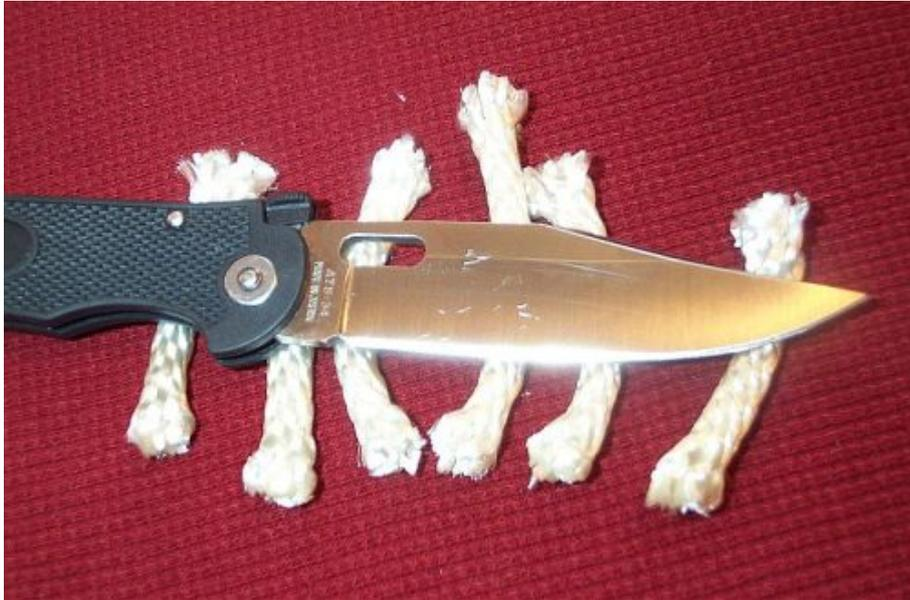
I expected that the AUS-8 would go easier, since it certainly seemed to pop hairs, especially after stropping with some green compound on cardboard. But something was wrong... the razor sharp edge just didn't seem to want to go thru the nylon, and when the cuts were completed the end was very frayed...
