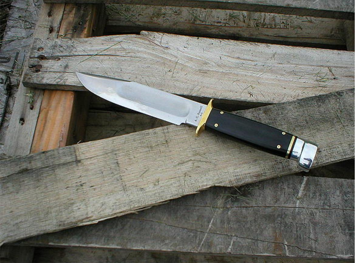
The Field Knife had more than sufficient strength to easily dismantle a few old pallets to scrap wood for my firepit. This knife won't come apart; the handle is pinned, epoxied, and the pommel is screwed on. It's one tough knife, for sure.
