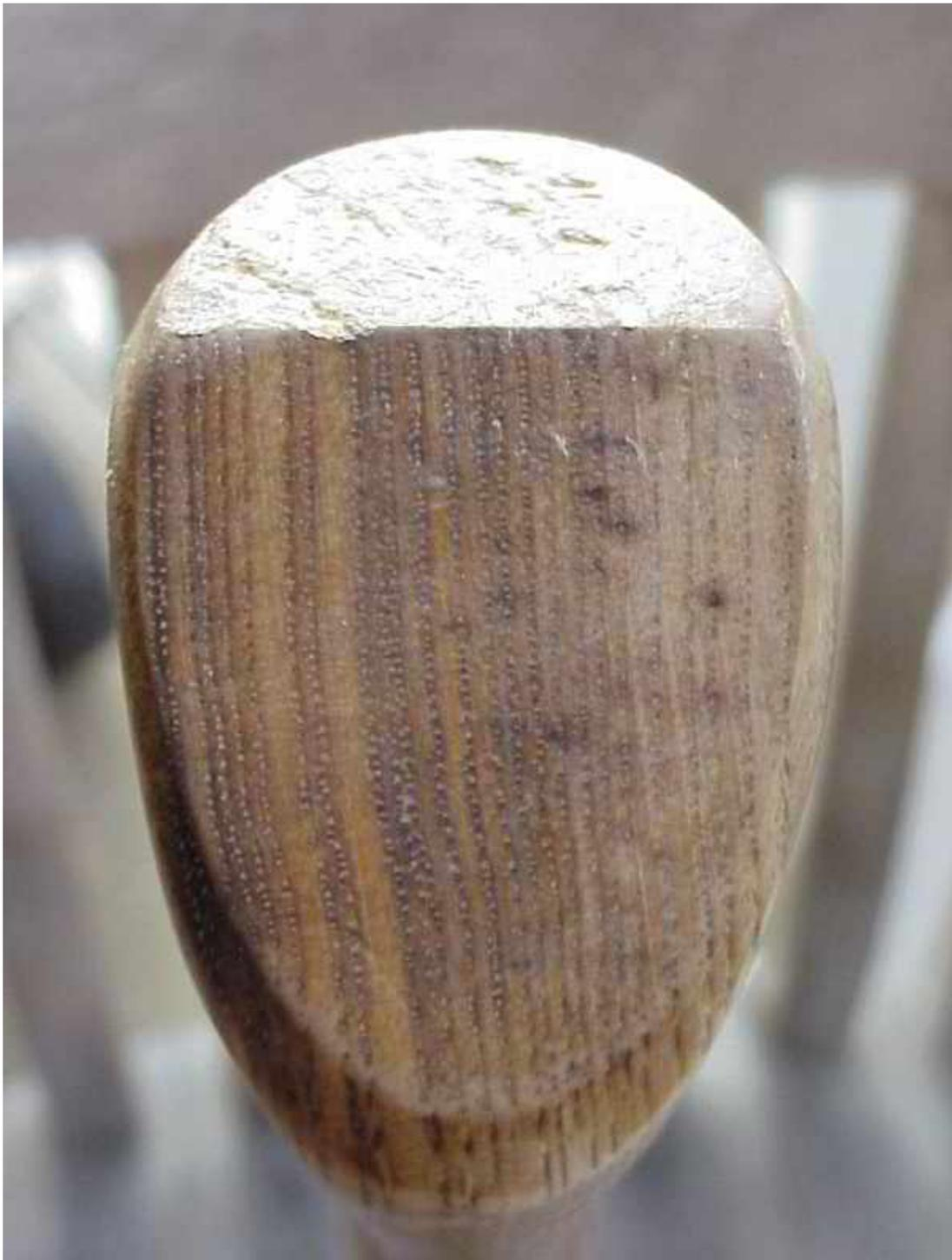
I got to choose from six. The one I got was the only one with anything like vertical grain in the handle, and it was also the only one where the head wasn't mis-aligned. The head is of good quality but the bevels didn't meet - instead someone had ground on a secondary bevel so that it would sort of feel sharp. It sure took some time on a belt sander to correct that. When I first used it, the head loosened on the second alder.
