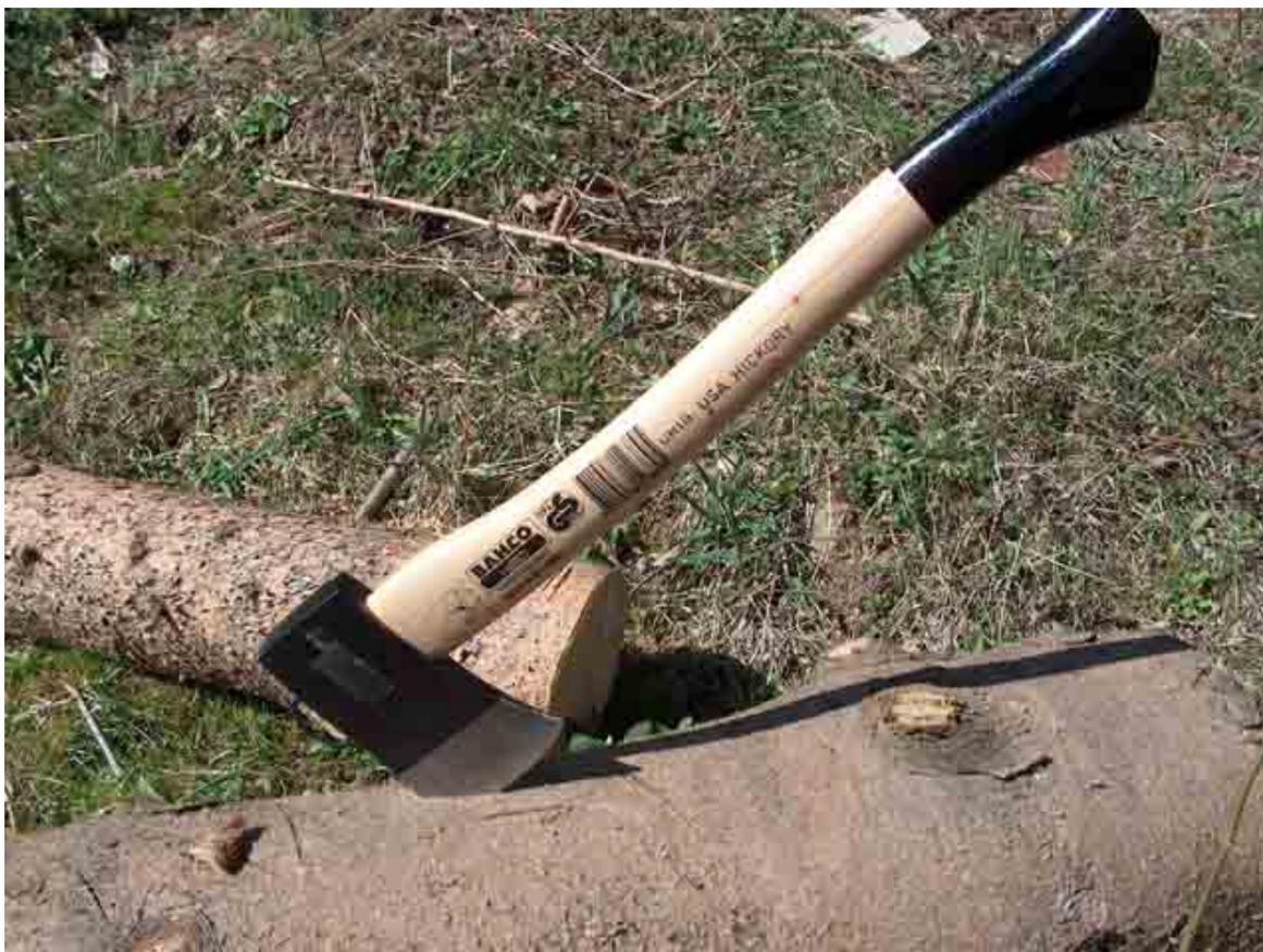
The only difference is that HUP models are professional ones, with handles from premium USA hickory and that HUP had an additional metal ring wedge together with carbon fiber one same as HUS model.
