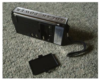
battery compartment Also visible are the headphone and adapter inlets.
