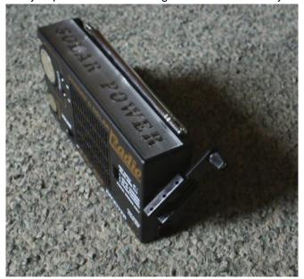
The hand crank In deployed mode. It folds up and stores a little more compact.
