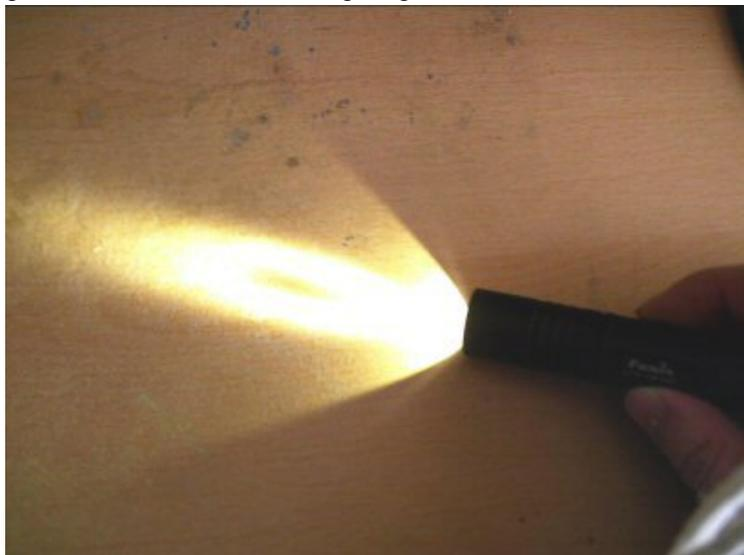
**Fenix L1P** the flashlight kicking out light, the donut hole in the middle is only visible at very very close ranges; 15 cm and closer.
