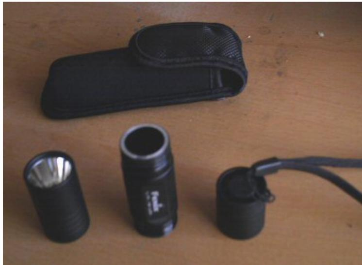
**the parts** sheath, head, middle section and tail.
