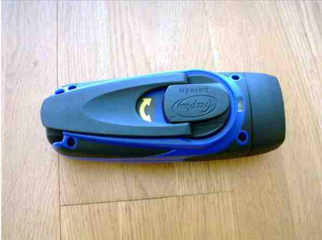
*The Freeplay Sherpa with crank unfolded. You can see the green led.*
