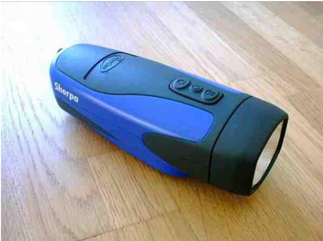
**BUT** get out of power, unplug the crank, wind it up 30 sec and you get 8 minutes of low power light, and some 45 seconds of high beam. You can also wind the crank from any beam mode.
