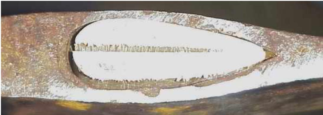
It's vital to go to work further scraping the handle to relieve the high spots that are causing this. Just go gently because you don't want to remove too much wood. It's probably just one high spot on the inside of the head, so look for where it is marking the handle. You may even want to blacken the handle with a marker or smoke from wet campfire wood to see the scrape mark better. **That comes later though, when you remove the axe head to saw the end to size.**
