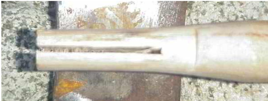
*I feel that this needs a little more fitting to bring the wedge slot no further back than the middle of the head where it holds tightest. ONLY file/sand/scrape the wood where it's compressed or marked by the head. The object is to get a fairly even contact. You slowly and patiently fit the head further and further back on the handle until no gap shows between the sides of the hole at the back and the handle.*
