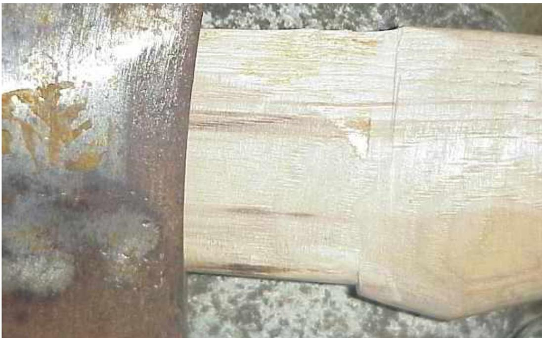
*Notice the spots smoothed and scraped by the head - just scrape or sand these to remove high spots. It'll get tempting to scrape more than you need to as you'll figure it'll mean less scraping later. Don't do it! The closer the fit the better.*
