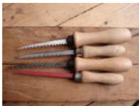
**The modified saws blades** Here are the tools I use for enlarging and fitting the tang hole.
