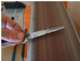
**Cutting and sanding the tang** Cut the tang to desired length, and send it using coarse grain.
