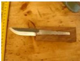
**Preparing the tang hole** Here we need to check the alignment of block and tang.
