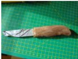
**Coarse shaping** Then, making progressive bevels, coarse grind the handle to the desired shape.
