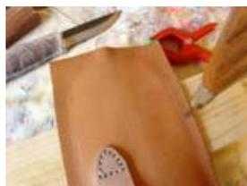
**Punch the holes** And we use the punch to make the holes.
