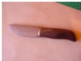
**The shaped block** I have shaped the wooden block to fit the blade.
