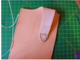
**Make the holes and prepare to stitch** Here I used a demmel for the holes, but a bladed leather punch does better.
