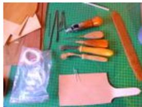
**Leather tools** Here are the tools and materials, thread, leather, punches, roulettes, the top most punch is a sewing punch.
