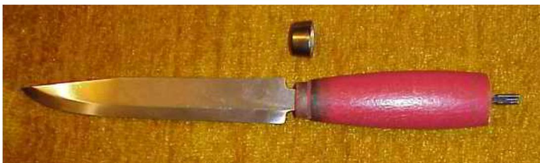
Here's a close up of the split collar. The hole for the last part of the tang is drilled to size, with a slightly larger hole drilled from the back to hold the split collar. There's not much holding the knife together. But it does hold together - we know that!
