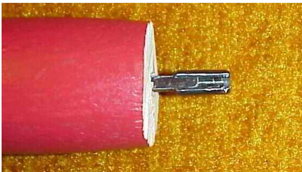
The last two pictures show the large round hole drilled in the front of the handle with sawed slots to take the wide front of the tang.
