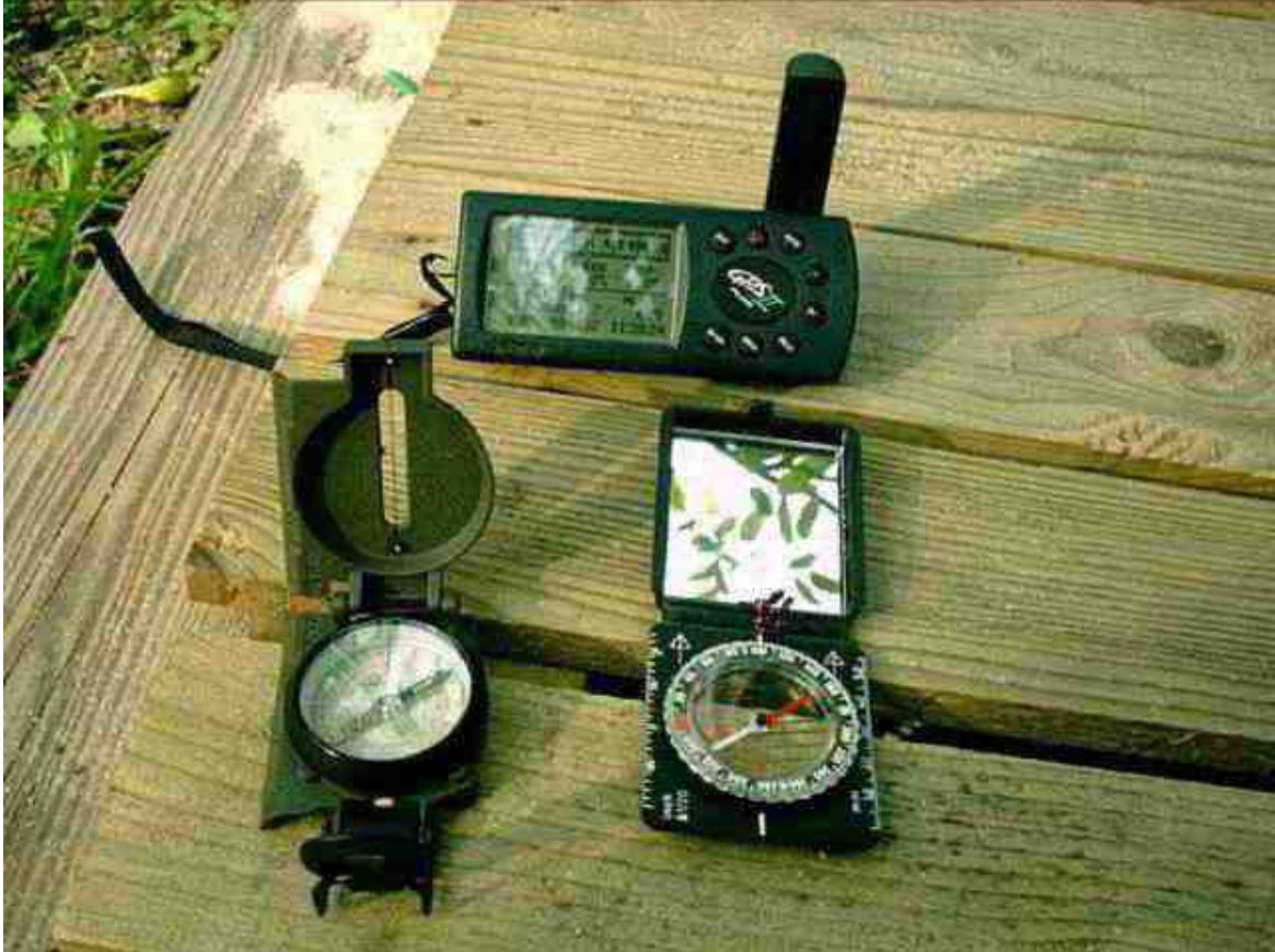
Garmin GPS II plus, Metallic compass with lens and wire sight, Silva plastic compass with mirror sight
