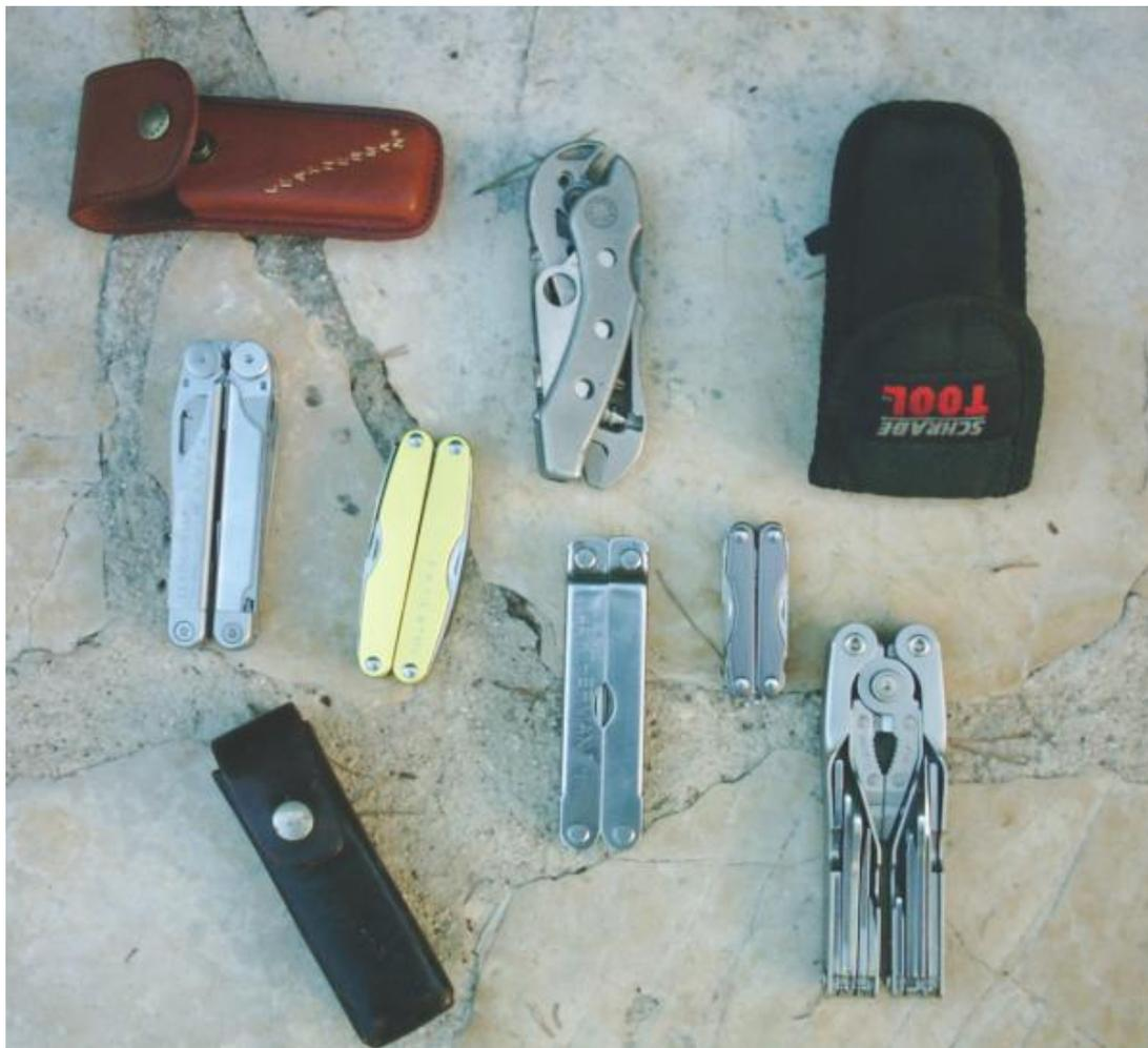
The comfort of the tool is an important consideration. With the first Leatherman, the handle would offer a very bad comfort, when using the pliers, because they form an open shell, and only the opening come in contact with the palm. More recent tools have changed the opening mechanism, or padded the sided of the handle to provide a surface for the palm to rest when using the tool. Try before buying.
