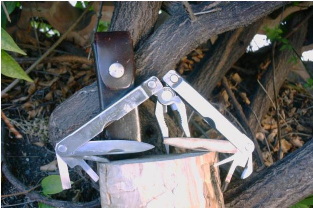
Leatherman built this inventive new pocket tool, a pair of needle nose pliers, whose handles fold around the nose, and contain additional tools like flat and Phillips screw drivers, a file, a knife blade, a can opener. While targeted at mechanics, these tools are really useful outdoors to repair any mechanical parts of modern gear, or cars.
