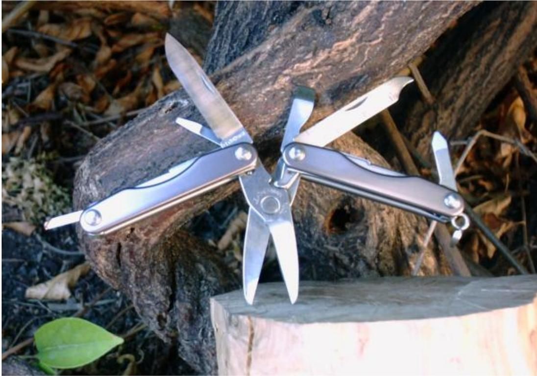
The big trend is to offer as many locking tools as possible, and direct access to a few blades when the pliers are folded (on most models you have to open the pliers to access the tools).
