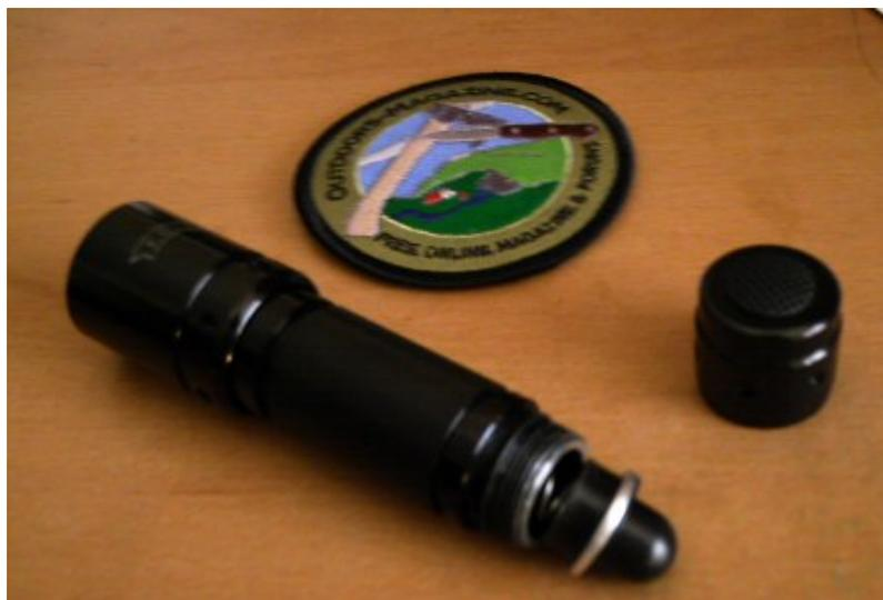
**the switch** The end removed and the metal disk with the spring and knob in place.
