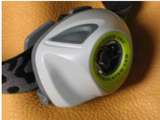
Note that some lettering has been removed- it smudges easily and then looks bad, so I just removed it entirely. I left the lettering that is recessed in the bezel. While operating the light, the first click goes to high, the next to medium, then low, and then a blinking signal mode. Leaving the light in any of the modes for a few seconds allows it to be turned off with the next click.
