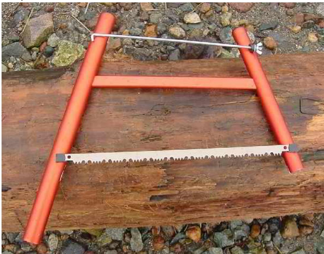
*The centre spacer only really fits one way. The tensioner rod is of course placed backwards - not to worry it only fits one way too, and that's easy to figure. The bottom line is that once you've fitted the saw together a couple of times and taken it apart and placed the components in the tube - you'll be able to assemble or disassemble blindfolded or in the dark. Well who knows? You might want to do some late night woodcutting..*
