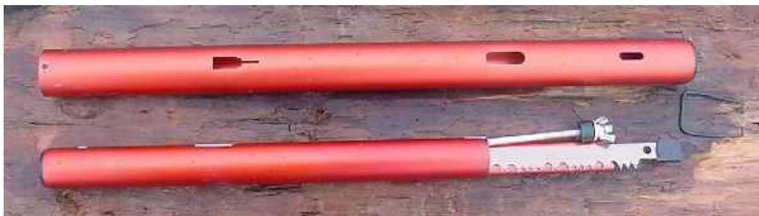
*This picture shows the common mistake of just putting the tensioner rod into the tube. By fitting it inside the rectangular tube spacer more room is left for extra blade.*
