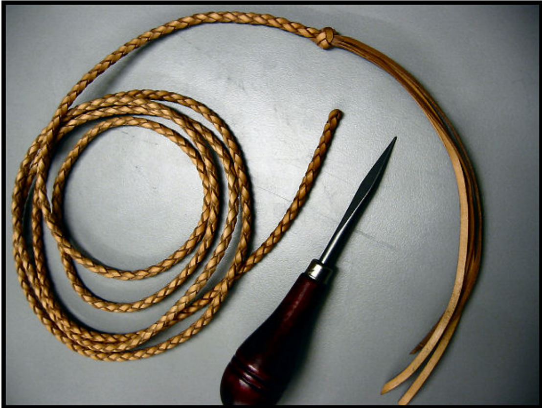
Finished 4-plait string Blunt end for stringing through the PSK knife handle holes.
