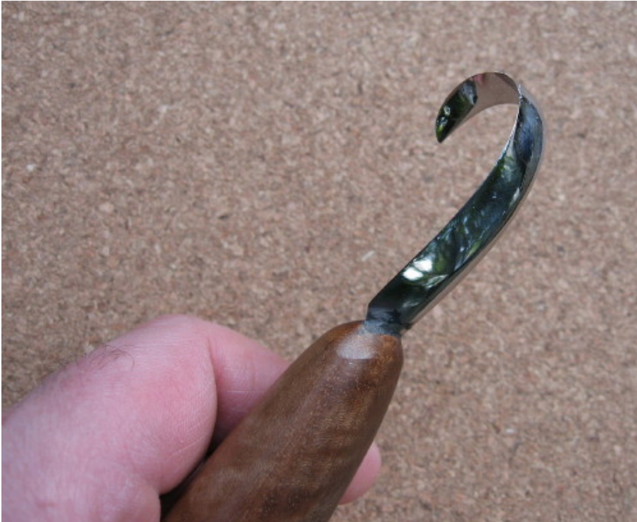
Dell Stubbs spoon knife, edge up The white spots on the edge are tiny basswood shavings
