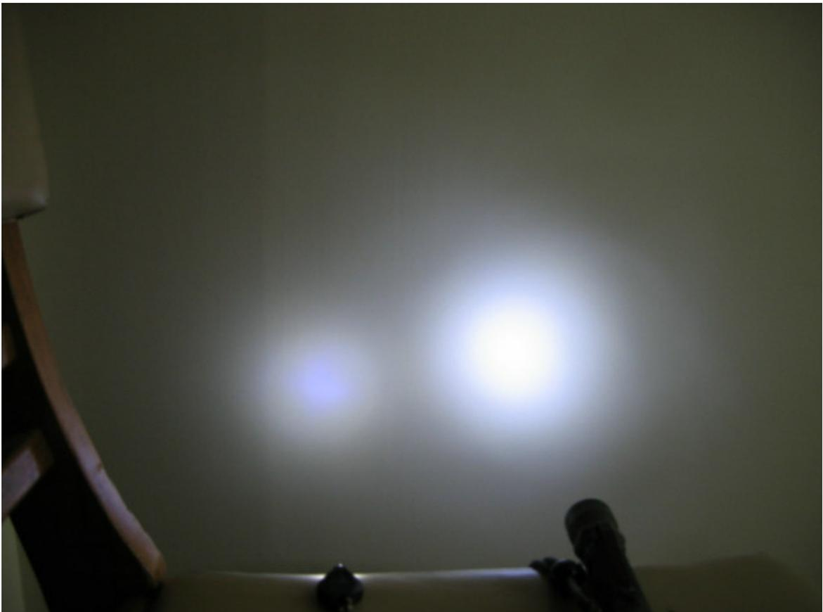
Beamshot with Aviator's LED's on right and Photon Freedom on left. The LEDs provide a nice flood, and their runtime is advertised as 20 hours. It is bright enough for many tasks, from reading to walking a path, thus lengthening the
