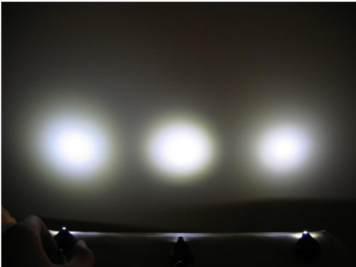
Left to right: New Photon, New Photon Covert, and Old Photon. I submerged my Photon in about 6 inches or water for a few minutes and found no water inside the case. It should survive most outdoors conditions just fine, but if water does get inside, just disassemble it, let it dry, and it should work just fine, with the possible exception of the batteries.
