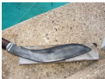
Temper line I am lucky, the best temper line I have met on a kukri.
