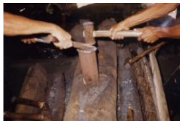
More forging And a better view of the very simple plug anvil
