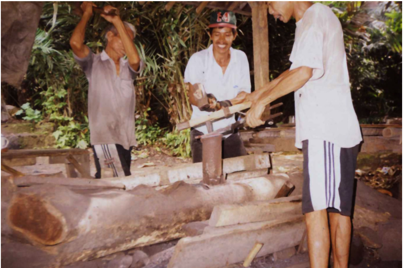
The smiths forging. Note the "plug anvil", a very elegant solution.
