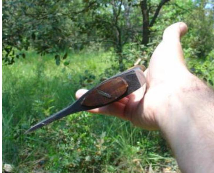
**The SFA balance and profile** The bit is too heavy compared with the poll. Note the hollow bit with a rather pronounced convex edge.
