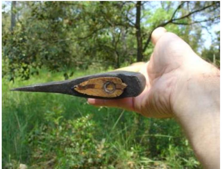
**The LHA balance and profile** The balance is perfect by Kochanski's test. Note the thin and reasonably straight profile.
