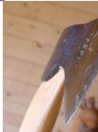
**LHA original sharpness** The secondary bevel can be seen
