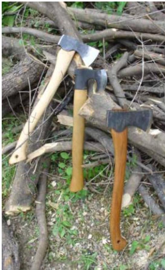
**Three axes.** Here during the tests on olive wood, cutting a good sized branch, you can see the test cuts behind each axe edge.
