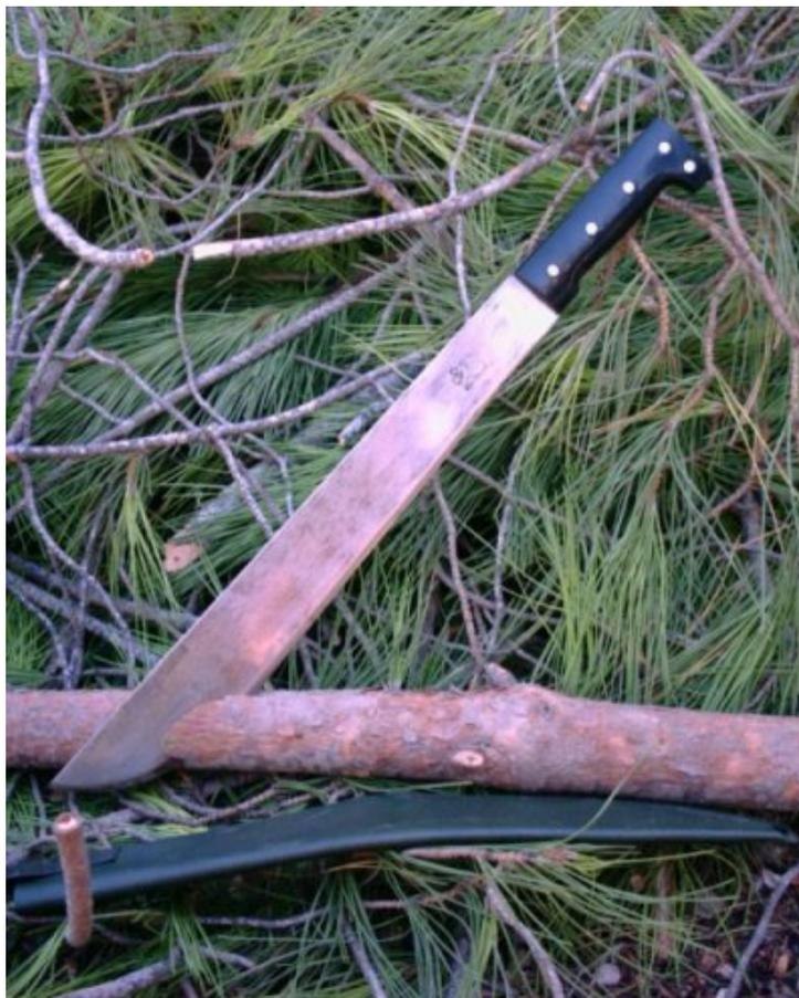
These are big bladed knives whose primary purpose is to clean vegetation, limb small trees, cut bamboo, and provide various cutting tasks adapted to rather tropical , equatorial, jungle or bush environments. Sizes there go from 10" (25cm) to more than 30" (75 cm) blades, depending on the tool specificities. Traditional asiatic blades do very well, but the classical south-american machete is also an excellent and cheap choice.
