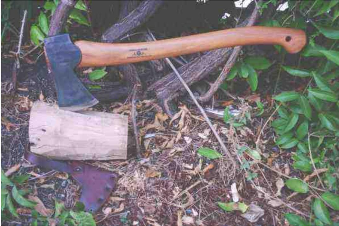
The axe is the (non-motorised) tool that provides the maximum power to fell or limb a tree. Axes sizes, and weights may differ widely, and their characteristics adapt to the type of work to do, from felling big trees to doing carpentry work, or even shaping wood. I like the [Gränsfors Bruks Small Forest Axe VS Roselli Long Axe](#). [[Axes](#)]
