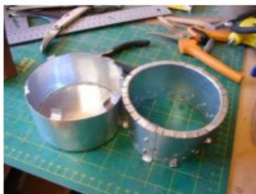
**The burning chamber** The burning chamber is finished and ready for final assembly. The inside wall is on the right, the outside wall and bottom on the left.
