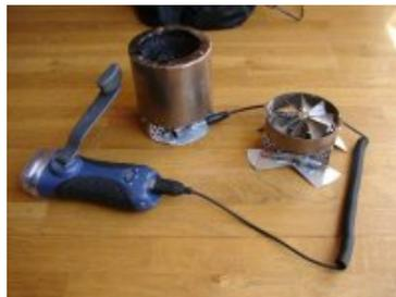
**an the last extra small modell** Here showing it's alternate power supply! This one piece model did not work very well, because of too thin walls, and was later rebuilt...
