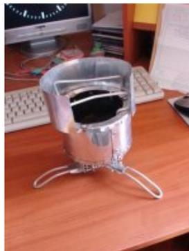
**A finished titanium model** The aluminium can holder burnt on second try... replaced by a titanium cross.
