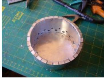
**The chamber assembled** And riveted. at the bottom of the inside wall, it is good to plan some folds, at a cm distance, to keep the spacing right.
