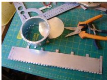
**Start assembling and folding.** Do that carefully. Remember to plan for the thickness of the sheets, 0.5mm is not insignificant.
