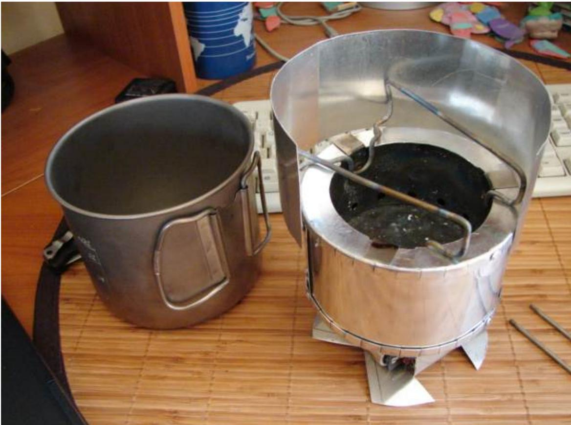
**And deployed** The pot rest bars are titanium.
