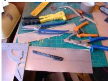
**Cut the different pieces to size** It is the first thing to do, following the plans, cut all metal to size.
